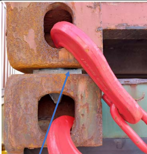
H-beam stopper welded between containers and tension levers
