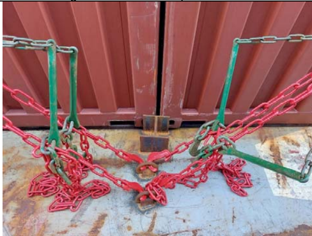
H-beam stoppers for corners post and pad eye for chain lashing welded on tank top/hatch covers/deck
